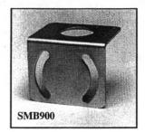
Accessory mounting bracket model SMB900 (left) has curved mounting slots for versatility in mounting and orientation. The sensor mounts to the bracket by its threaded base, using a jam nut and lockwasher (both included). The bracket material is 11-gauge zinc-plated steel. The curved
